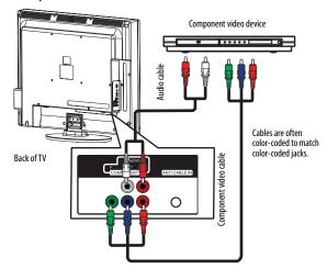
3 Connect an audio cable (not provided) to the L and R audio jacks on the back of your TV and to the L/R AUDIO OUT jacks on the component video device.
